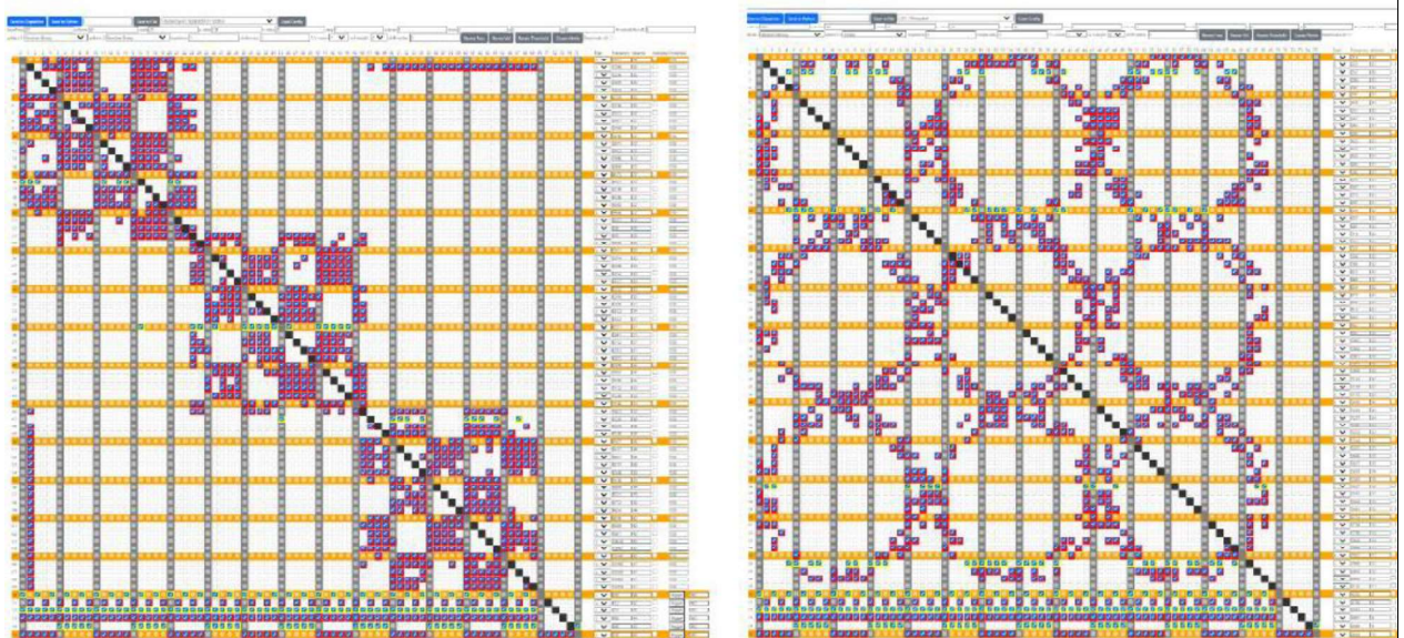
Figure 22: Connectivity matrix with a circular pattern (right) or three loosely interconnected subnetworks based on a checkerboard pattern (left). Each row encodes a transmitting neuron and a column a receiving neuron
